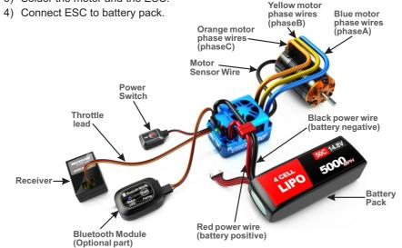
You may use the mounting plate(included) to fix the ESC to the chassis.
